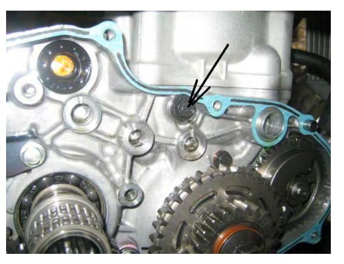
Must refit this bolt if removing e-start components. (oil transfer issue if not re-fitted) Pack out with washers to prevent original bolt going too deep into case!
