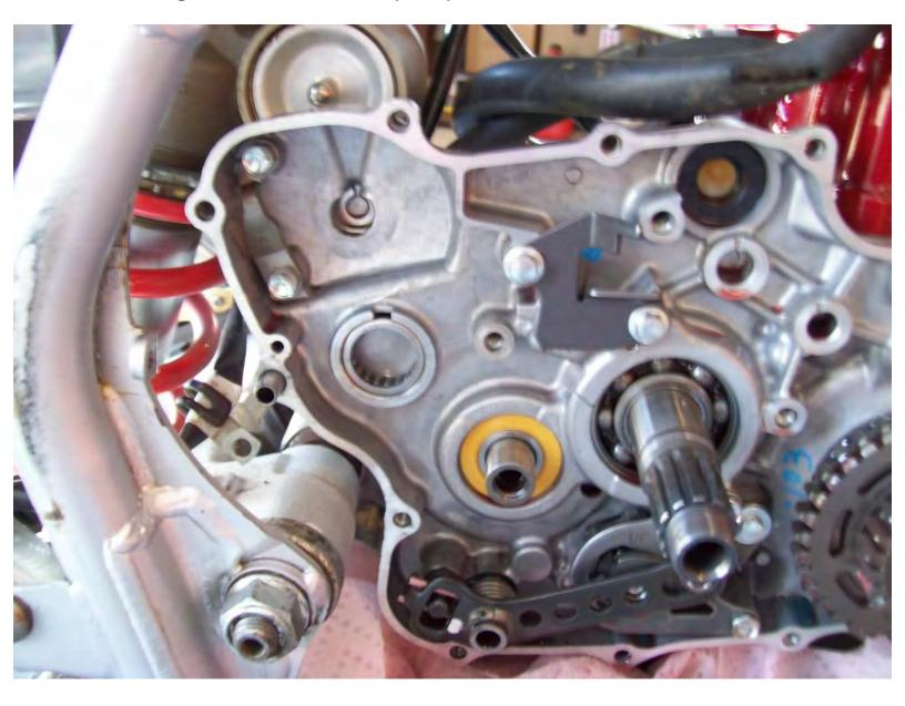
17. Assembly of the kick start shaft, take 10..SPINDLE and slide 16..WASHER (20MM) onto the shorter side, take 02..PINION (28T) and slide it on the same side followed by 16..WASHER (20MM), take 20..CIRCLIP (19MM) and snap it into place on the same side, take 04..RATCHET line up the punch marks and slide it on the same side, lastly 05..SPRING goes on. Next slide 11..SPRING onto the long side of the spindle, the spring goes into the hole in the spindle, then slide 12..COLLAR over the spindle.
