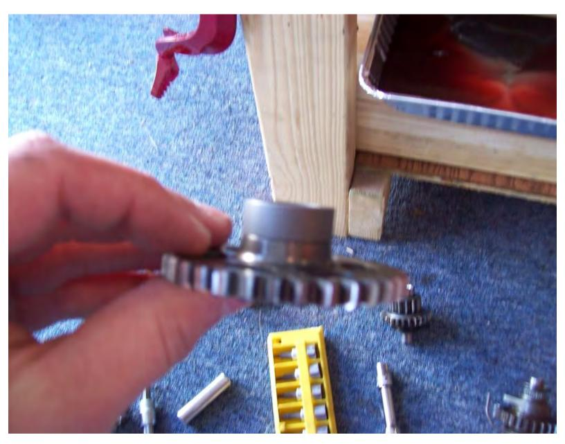
12. Install that assembly onto the yellow bearing in the case 13. Install 08..PLATE to hold the idler gear assembly on
