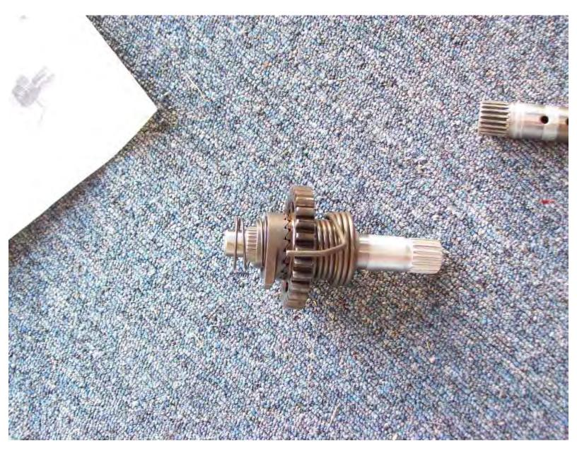
18. Slide the whole assembly into the hole in the top left of the center case. Then rotate it so the part that sticks out on the ratchet will slide behind the stopper plate. Then pull the spring into the hole on the case
