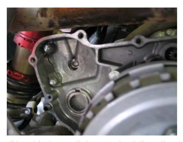
Kick start shaft and gear assembly, there are several parts in this assembly so referencing the service manual is recommended. (Exploded view of all the parts and the order installed)
