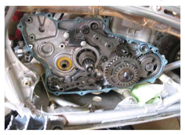
Install the gear on the collar then install the gear/collar onto the end of the countershaft then install the stopper plate.
