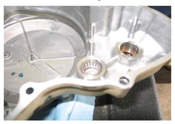
Remove the clutch and basket assembly to install the kick start idle gear.
