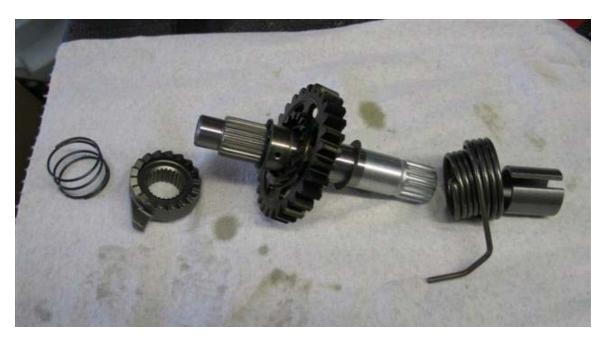
Install the kick start shaft gear assembly into the right side center case then rotate the recoil spring counter clockwise and put the end into the hole in the case above where the dowel pin is located this will lock and hold it in place.
