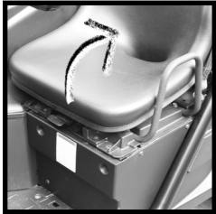
Remove both seats easily by lifting the release lever under each seat.
