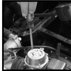
Remove the two screws from the gold colored carburetor diaphragm cover.
