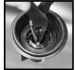
Using long-nose pliers, gently grasp and remove the needle keeper.
