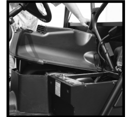
Reinstall the center console as shown. Pay close attention to the next photo...
