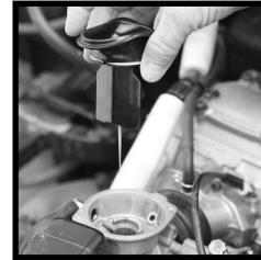
Gently lift and remove the rubber diaphragm. Check for tears and replace if necessary.
