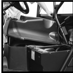
Lift and remove the center console between the two seats.
