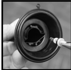
Place the needle back into the diaphragm and reinsert the needle keeper as shown.
