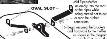
16) Begin securing the brackets and hardware to the muffler as shown in the diagram at left. First, insert the rubber spacer into the muffler bracket followed by the aluminum axle/sleeve.
